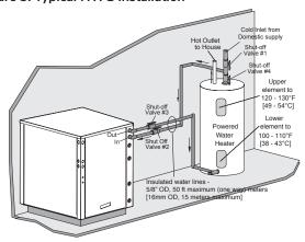
Using a 125°F setpoint, the HWG can heat the lower 40 gallons of water from 100°F to 125°F, providing up to 8,330 btu's of heat. Using the 150°F setpoint, the HWG can heat the same 40 gallons of water from 100°F to 150°F and the remaining 10 gallons of water from 125°F to 150°F, providing a total of up to 18,743 btu's of heat, or more than twice as much heat as when using the 125°F setpoint.
